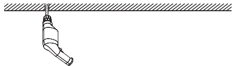
1. Drill a \varnothing 6\text{mm} hole
